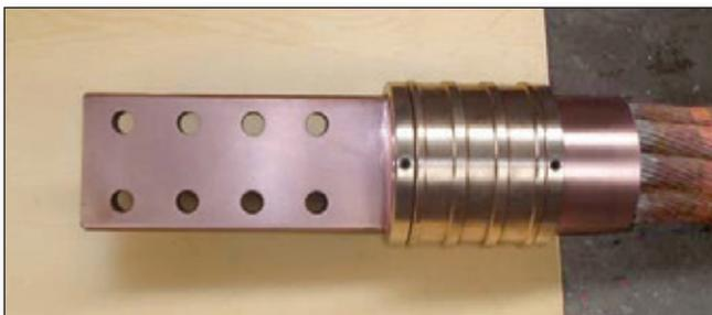
Using a rotating terminal at one end of the cable reduces the stress on the hose during roof swiveling.
